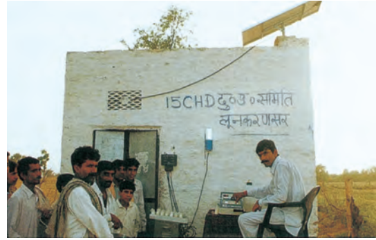
Fig. 5.11: Solar operated electronic milk testing equipment
